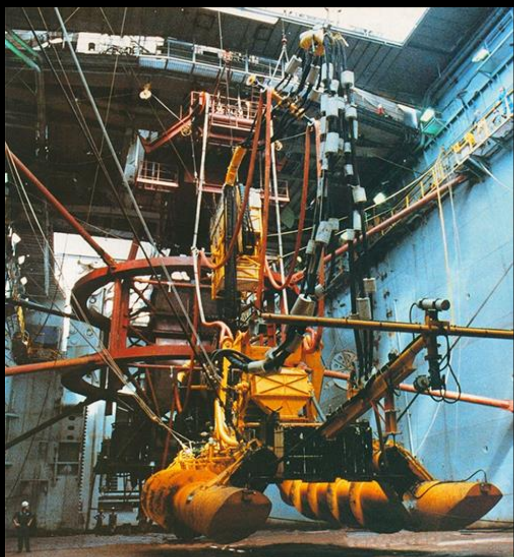
Figure 1: Prototype mining machine used for nodule collection at the OMCO site in 1979 (Credit: Lockheed Martin).
